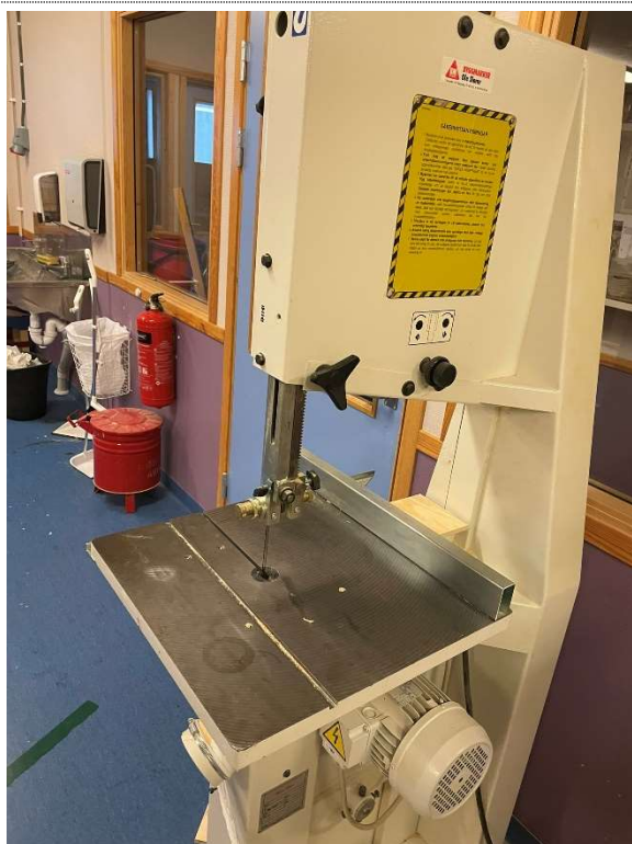
68 Inventar. Mangler sikring/deksel.
